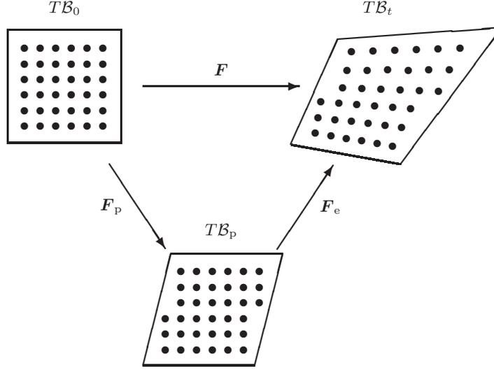
Figure 1: Basic kinematics: material isomorphism and its relation to the so-called multiplicative decomposition.
