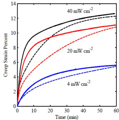
Figure 5. Photo-induced, nominal creep strain percents from model predictions (dashed lines) and corresponding experiments (solid lines) for specimens subjected to 500 kPa nominal stress and intensities of 40 (black), 20 (red), and 4 (blue)  $\text{mW cm}^{-2}$ .
