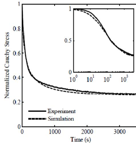
Figure 3. Model fit to a 6% nominal strain, 40  $\text{mW cm}^{-2}$  induced stress-relaxation experiment. The inset shows the same data with the time axis presented on a logarithmic scale
