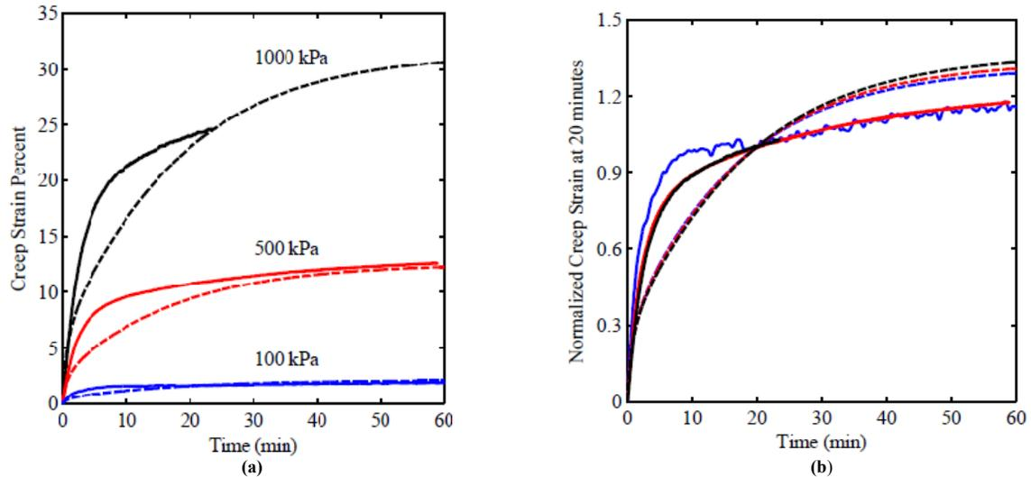
Figure 6. a) Photo-induced, nominal creep strain percents from model predictions (dashed lines) and corresponding experiments (solid lines) specimens subjected to 100, 500, and 1000 kPa nominal stresses and an intensity of  $40 \text{ mW cm}^{-2}$ . b) 100 (blue), 500 (red), and 1000 kPa (black) creep curves normalized by their respective values at 20 minutes.
